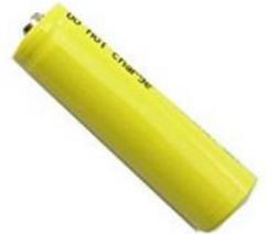
Unlike the FT-60 which can handle voltages from 9v to 6v, a Baofeng won't transmit if the battery voltage is higher than about 8v.
